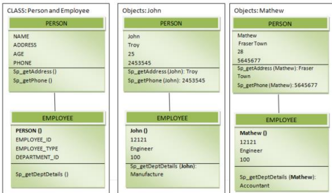
Figure 4.4: Object Data Model Example
